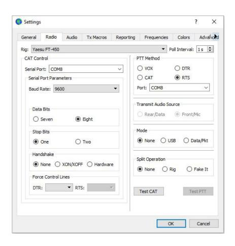
On the RigBlaster set the switch to "COM" If all has gone well, the "TEST CAT" should turn green.. Gary/MOTIG
